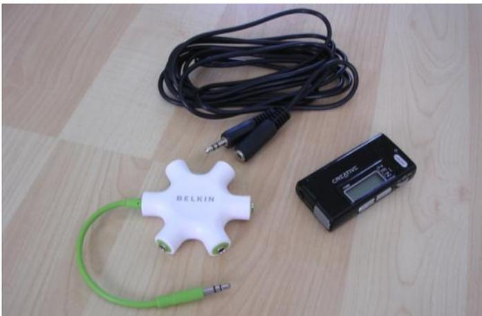
Figure 7: Audio multi splitter (Rockstar, Belkin), audio recorder (Zen Nano Plus), audio extension cable.
