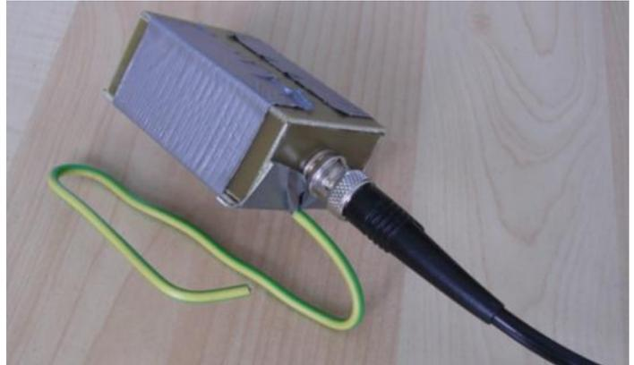
Figure 5 b: Home constructed LPF: Filter box.
