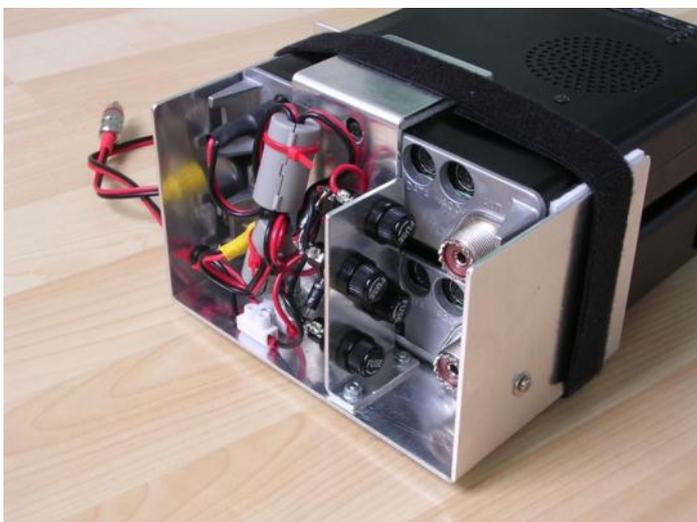
Figure 3 b: FT-817NDs in the transceivers box: Bare box from back with all parts mounted.
