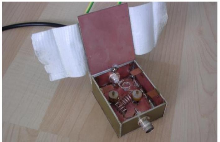
Figure 5 c: Home constructed LPF: inside of the filter box.
