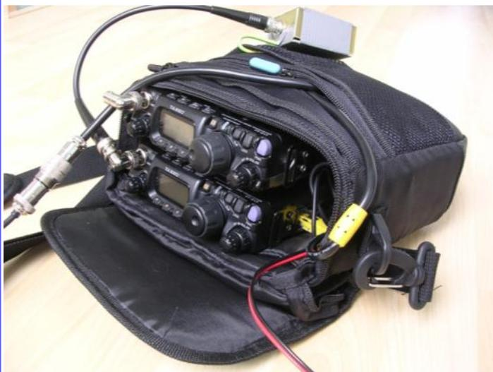
Figure 3 d: FT-817NDs in the transceivers box: Box mounted in carrying bag, space for audio cables visible, LPF clipped onto carrying bag.
