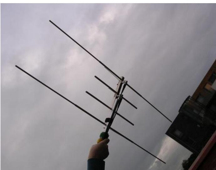
Figure 4: HB9CV dual band 2 m/70 cm portable antenna.
