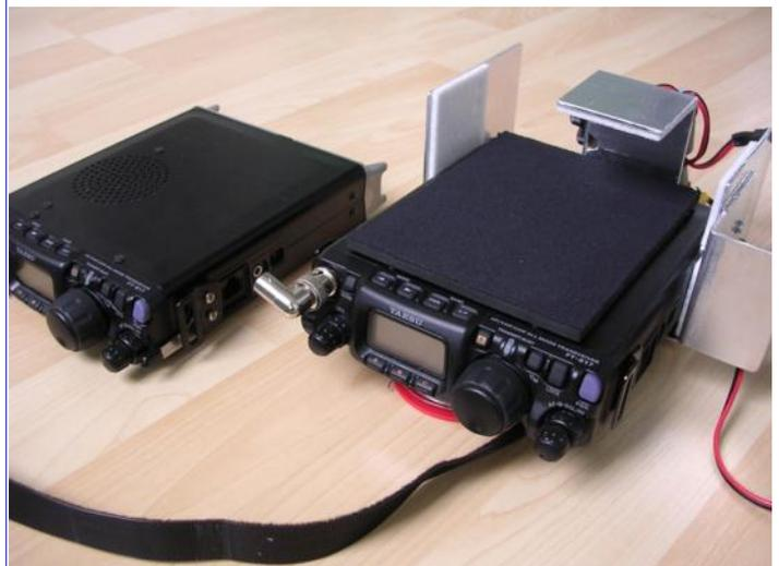
Figure 3 a: FT-817NDs in the transceivers box: Bare box from front with the bottom FT-817ND mounted.
